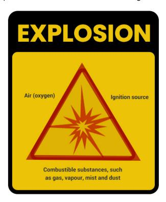
There are three factors will make it possible for a real explosion, even through we can take some measures to avoid the formation of explosive atmospheres, the leaked combustible substance still present probably, so Combustible substances, such as gas, vapor, mist and dust may exist, besides, we are impossible to avoid Air (oxygen) in any environment, so what we can only do to avoid explosion is only to control Ignition source.
